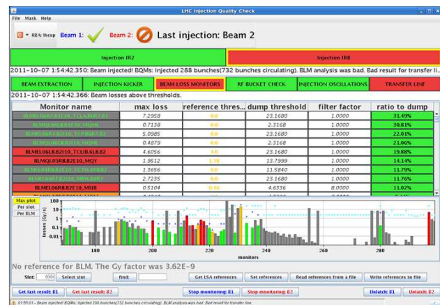
Figure 1: Losses in the LHC injection region for the first B2 288 bunch injection.
