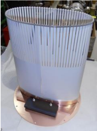
Figure 8: New assembly of the VMTSA module with the ferrite blocks.
