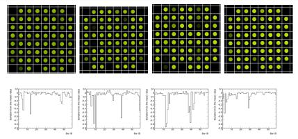
The plots show the deviation of the average luminosity of every channel from the mean value of luminosity calculated from 20 the most brightest channels. Downward spikes represents broken channels and the depth indicates the level of damage.
