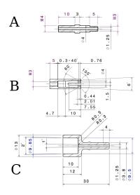
The part A (aluminium) is attached to the scintillator bar on both ends after the WLS fiber is inserted into the hole inside the bar and glued. After the glue is fixed, the end face of the part A is polished. The adapter B (plastic) is screwed onto part A and the connector C (plastic) is clipped into adapter B. The end face of connector C should be also polished. The enlargement in connector C will be explained later.
