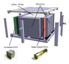
EMR detector is designed to fully stop muons from the MICE cooling channel and provide distinct signatures for muons and electrons.
