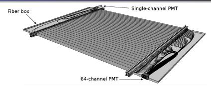
In the original design of the detector a 3 meter wavelength shifting fiber collects and transfers light to PMTs on both sides of a plane.
