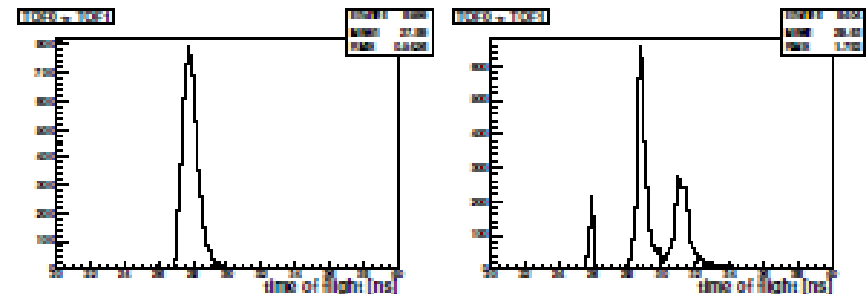
Fig. 10. Time of flight between TOF0 and TOF2 for muon (left) and electron (right) beam.
