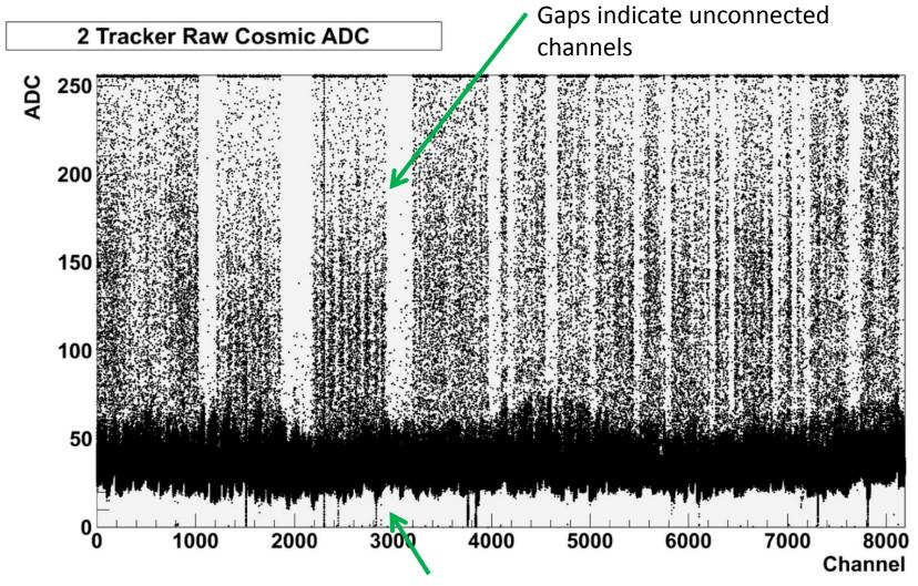
Lower spikes indicate channels in breakdown
