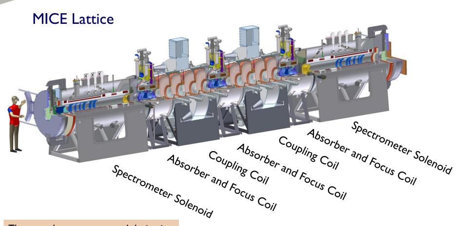
These are large magnets and design is complicated by the interaction (forces) from the rest of the MICE lattice in the various stages of construction.
