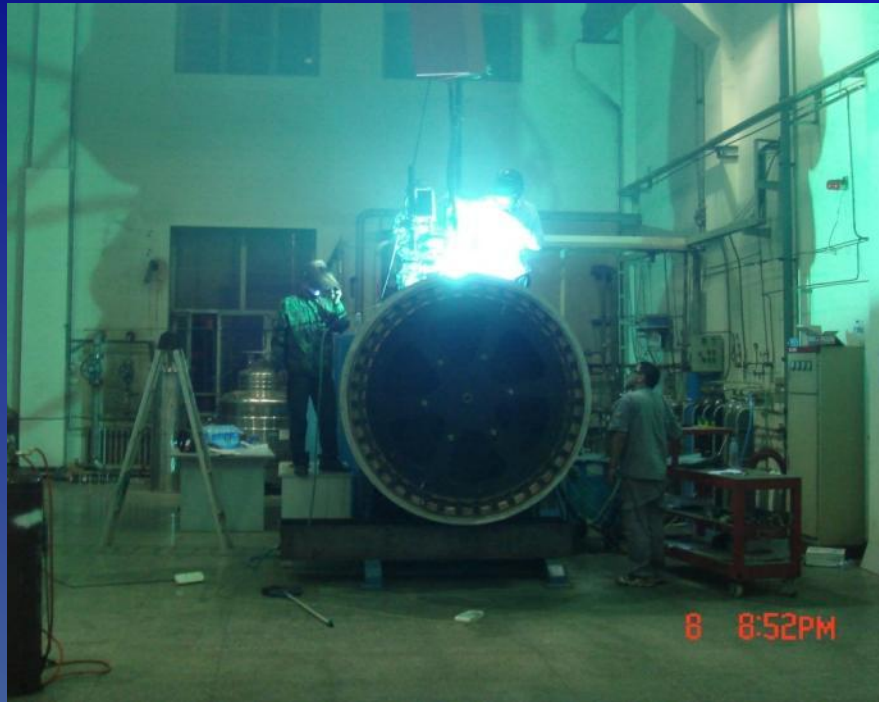
Cover plate welding at HIT in early August 2011
