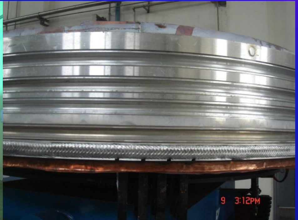
Cover plate welding at HIT in early August 2011
