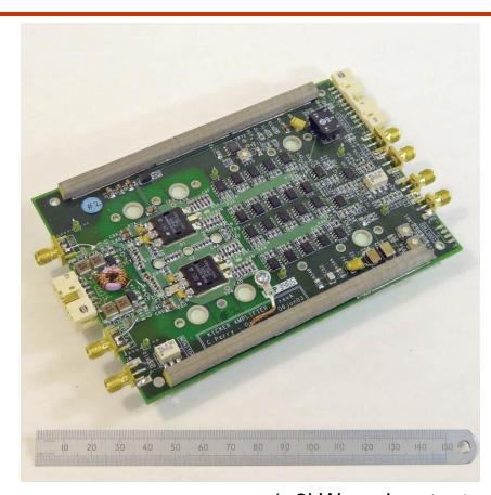
A 2kW peak output 10ns amplifier module
