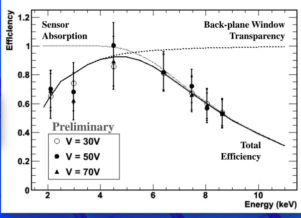
Extract equivalent thickness of backplane entrance window by 1-par  $\chi^2$  fit to measured efficiency curve:  $(0.6\pm0.2)\mu m$  of equivalent Si thickness, in agreement with result of SRA analysis.
