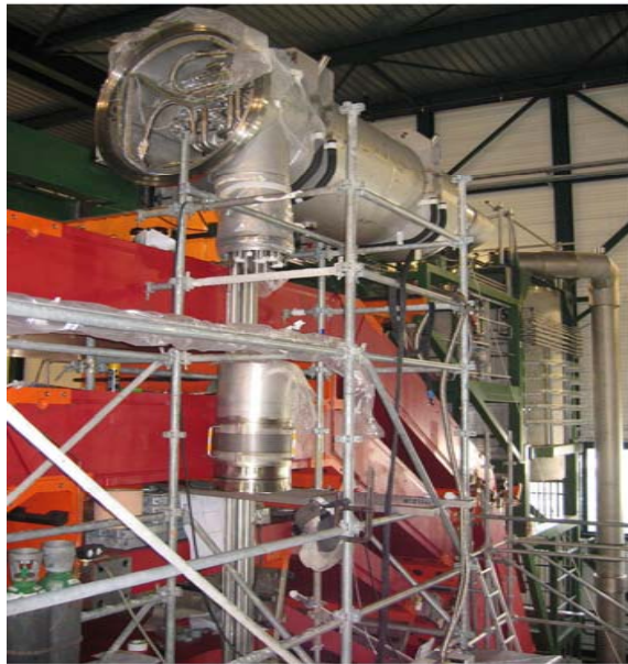
The cryogenic chimney links the cold mass to the phase separator cryostat by SDMS (F)
