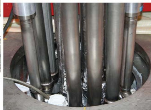
The cryogenic chimney links the cold mass to the phase separator cryostat by SDMS (F)
