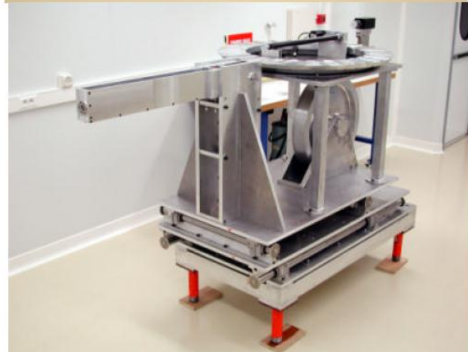
"Carousel" brick dispensing and storage system
