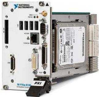
Embedded Controller (Processor)
