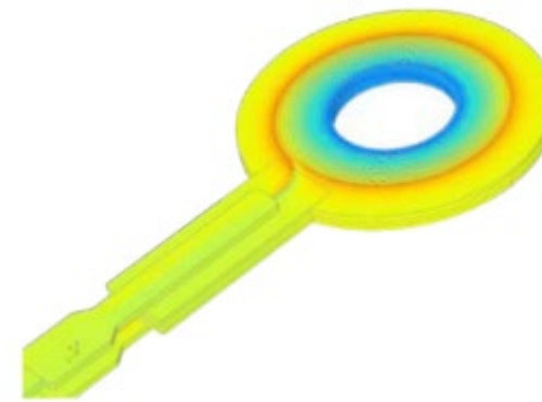
EM simulation of a NINT coil
