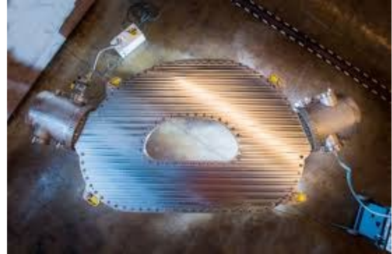
SPARC TFMC 2021 – Previously World's Largest Highest Field Pure HTS Magnet (20T)
