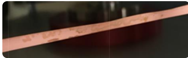
Unwound tape with plastified edge.
