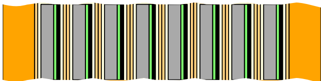
Removing the low resistance radial path: removing the coil's sides.
