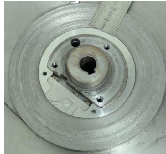
Sub-coil Geometry – dimensions of the superconducting pancake: 6 cm ID, 10 cm OD, 4 mm high
