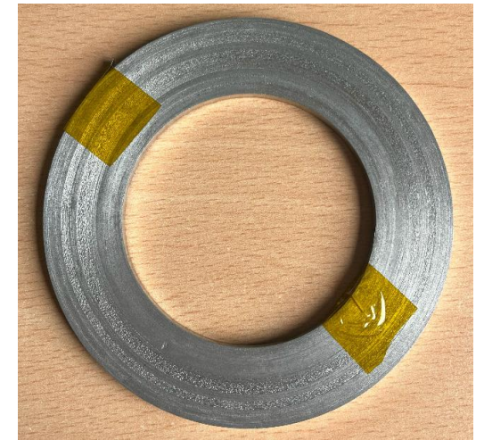
Sub-coil Geometry – dimensions of the superconducting pancake: 6 cm ID, 10 cm OD, 4 mm high
