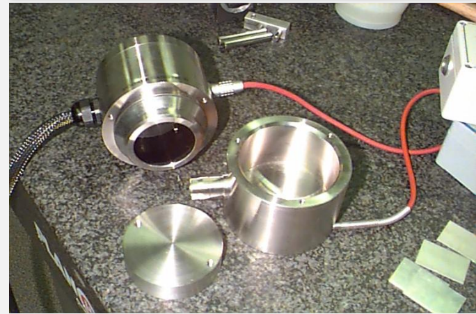
Typical HLS Pot and a previous installation
