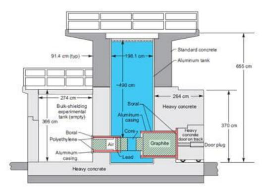
Reactor: 250 kW maximum power, can be regulated to few W. Total flux at maximum power is  $4x10^{12}$  cm<sup>-2</sup>s<sup>-1</sup> (central channel). NIEL (in Si) damage constant is 0.9 for fast neutrons. Several in-core and ex-core irradiation channels Maximum uninterrupted irradiation time is 16h. All irradiations done in two irradiation tubes. Accuracy of fluence is  $\pm$  10%
