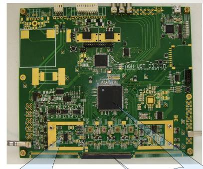
•32 channels fully equipped channels (Front-end +ADC)
