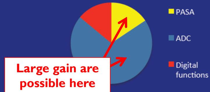
It is clear that the ADC power consumption limits the design to small channels counts.
