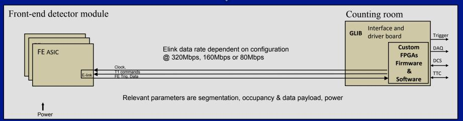
Considered as a continuous data stream output from the FE to counting room. We are free to choose our data packet structure.
