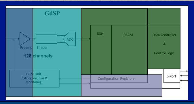
Preamp > Reduce current via bias control, important to maintain a low impedance on the electrode.
