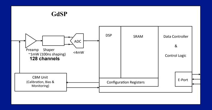
128 channels = Analog power 640mW + Digital power ~ some hundreds mW. Approx. ~900mW / chip.
