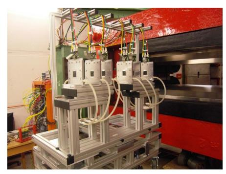
High resolution beam telescope (3µm) based on monolithic active pixel sensors was developed within the EUDET collaboration and optimised for the use at the low energy electron beam at DESY.
