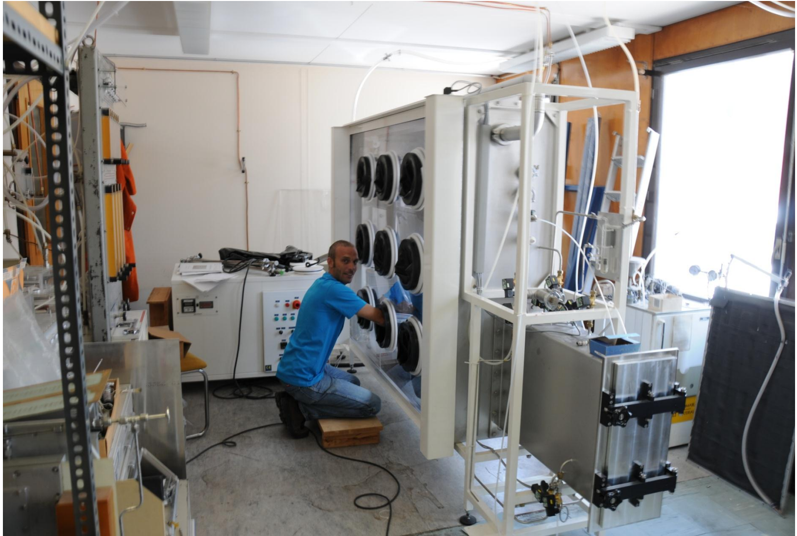
Six triple TGEMs were assembled using a glow box inside the RICH prototypes gas chamber.
