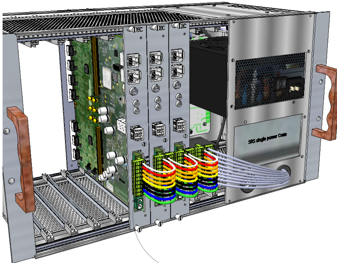
Power cable bus for 4 Combos
