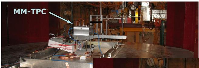
~20x20x10 cm<sup>3</sup>, 1cm thick aluminum box, 10 cm in drift direction
