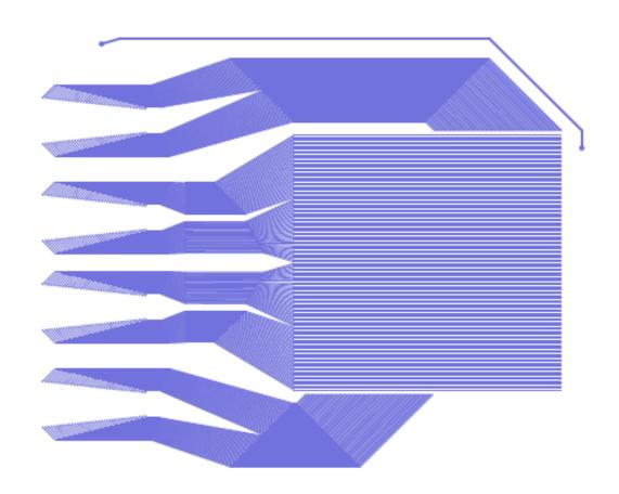
Based on MIMAC's Saclay design modified and constructed by Rui's lab at CERN. 2x144 strips, ~700 µm pitch
