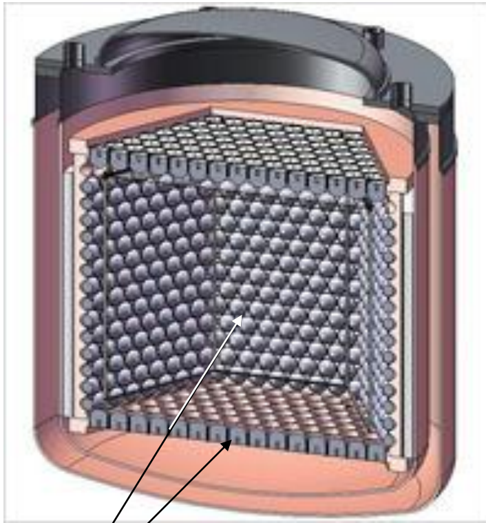
Large amount of PMs in the case of the large-volume detector significantly increase its cost
