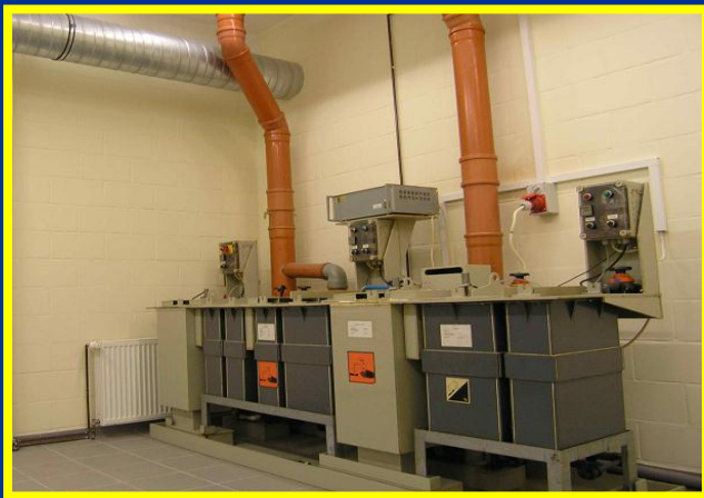
Kapton etching device moved from Eldos to WPT.
