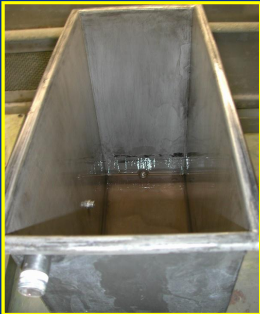
Single-jet acid etching bath, CERN.
