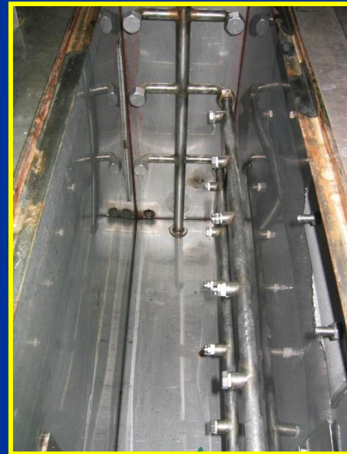
Multi-jet acid etching bath, Techtra
