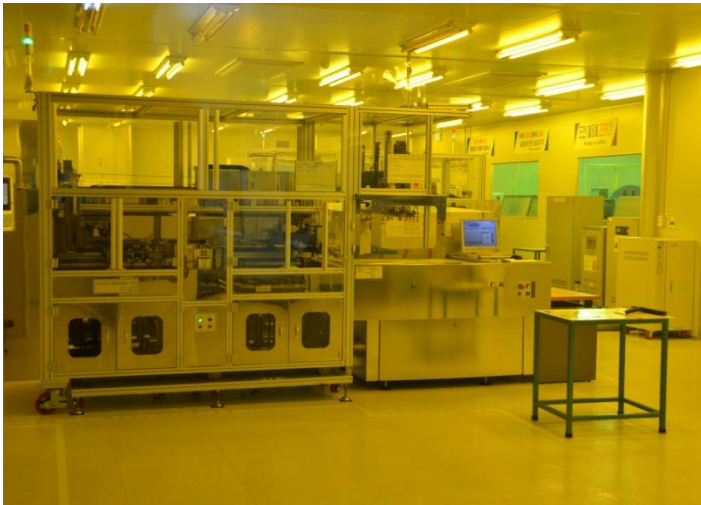
Production line Laser Direct Imaging (LDI) with automated charger (CERN has the same but manual)
