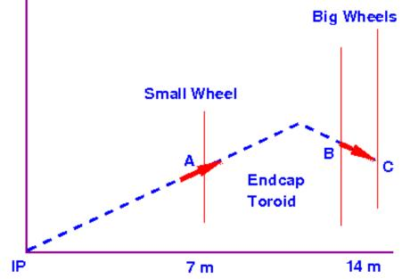
ProposedTrigger Provide vector A at Small Wheel Powerful constraint for real tracks With pointing resolution of 1 mrad it will also improve pT resolution Currently 96% of High pT triggers have no track associated with them
