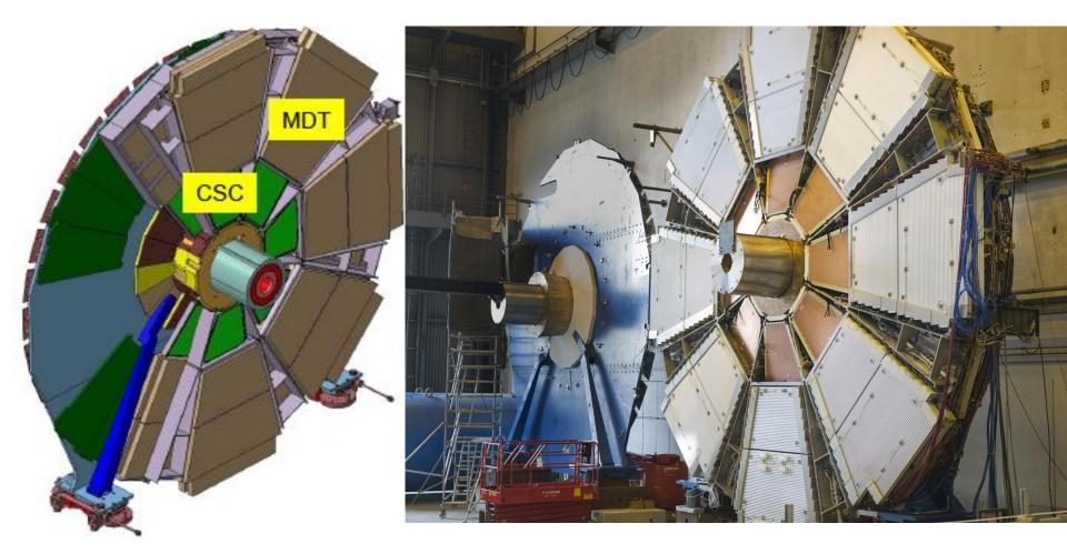
Need New Detectors that participate in the Level1 Trigger by providing a vector with ~1 mrad resolution
