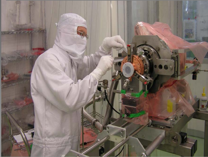
Cathode cooling unit assembly
