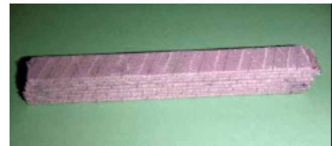
Heat-treated conductor stack with CEA innovative insulation (Courtesy F. Rondeaux & P. Fourcade, CEA)
