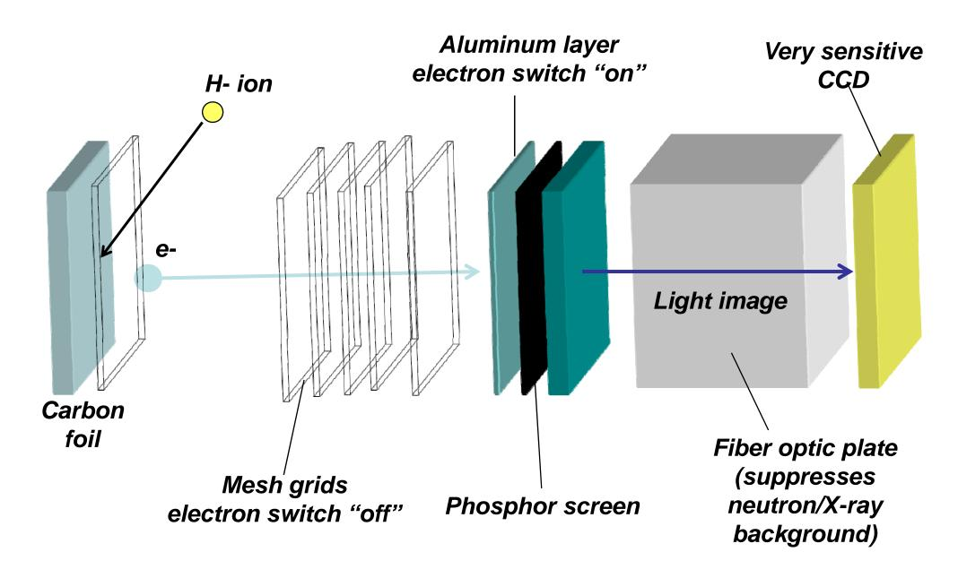
9-electrode configuration, increased distances between grids, no initial acceleration, no B-field
