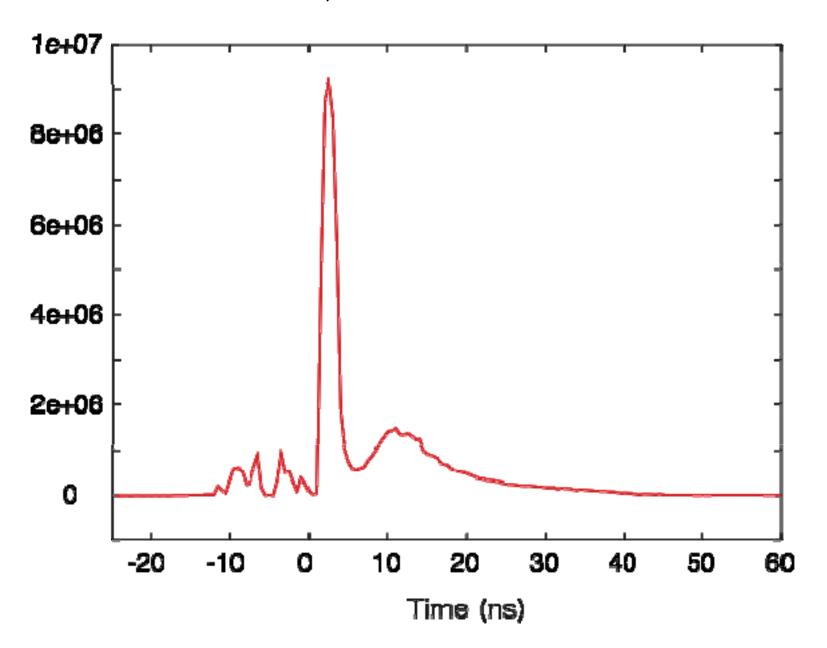
10-electrode configuration, kV initial acceleration, no B-field sweeping electrons.
