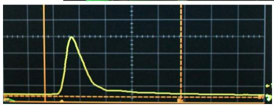
SBS process to compress Nd:YAG laser pulses to < 500 ps (trace 1 ns / division)
