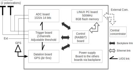
•1 ADC board: 14 bits waveform. 1GS/s,  $2.5 \mu s$ , 1-250 MHz BW
