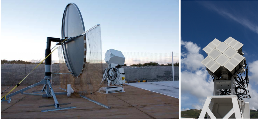
FIGURE 1. The AMBER (Air-shower Microwave Bremsstrahlung Experimental Radiometer) telescope is installed alongside the High Elevation Auger Telescopes (HEAT). The 2.5 m parabolic dish (left) is instrumented with a 16 pixel camera (right).
