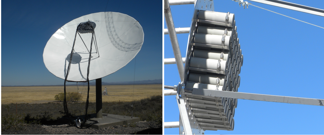
FIGURE 3. MIDAS (Microwave Detection of Air Showers) uses a 5 m parabolic dish (left) instrumented with a 53 channel camera (right) and is installed at one of the FD sites.
