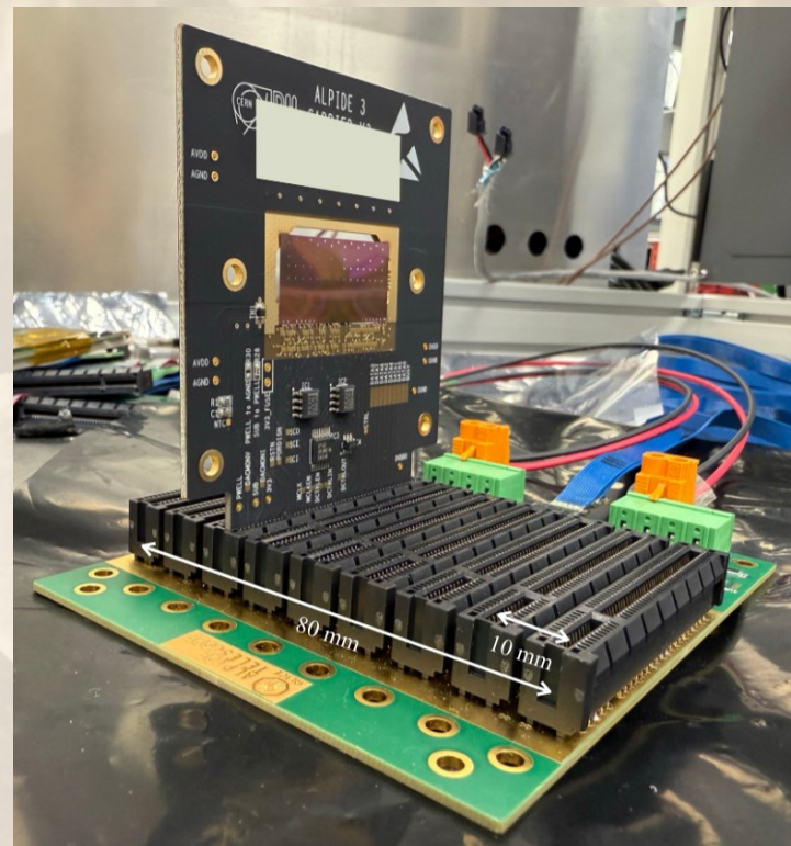
9-chip adapter board with one mounted carrier board
