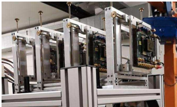
Test beam with HV-MAPS tracking station (MuPix8)
