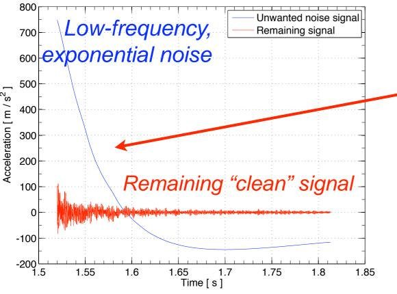
Wavelet decomposition can be efficiently used to subtract the "slow" baseline modulation (oscillation + exponential decay)
