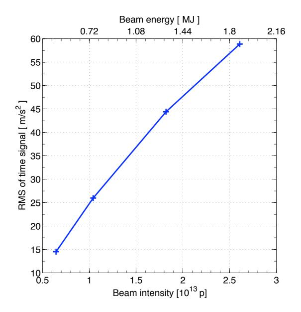
Expected scaling against basic beam parameters (beam energy and intensity, impact parameter) is qualitatively confirmed!
