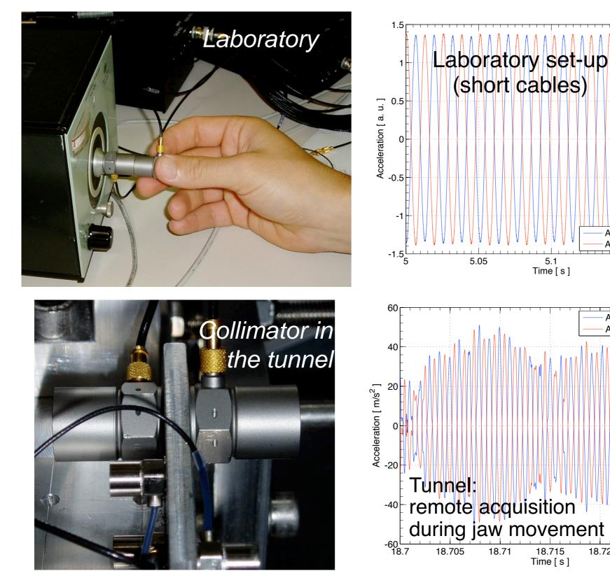
Verify amplitude and phase of two signals: for real vibrations, the two must sensors satisfy:  $A_1(t) = -A_2(t)$
