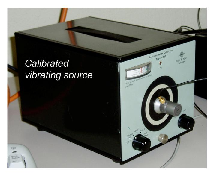
Calibration of the accelerometers was verified in the lab by means of a calibrated vibrating surface: Controlled acceleration of 1 g at 79.5 Hz.
