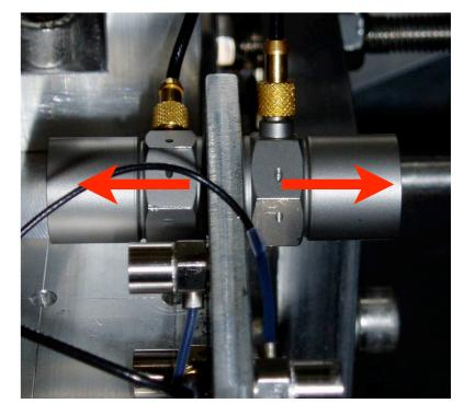
Calibration: for real vibrations opposite signals are expected. Expected behaviour found in the oscillations around the baseline (noise would be different!): we see real vibrations!
