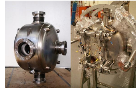
SC 5 cell cavity for 704 MHz, CEA and CNRS
