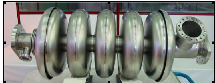
SC 5 cell cavity for 704 MHz, CEA and CNRS
