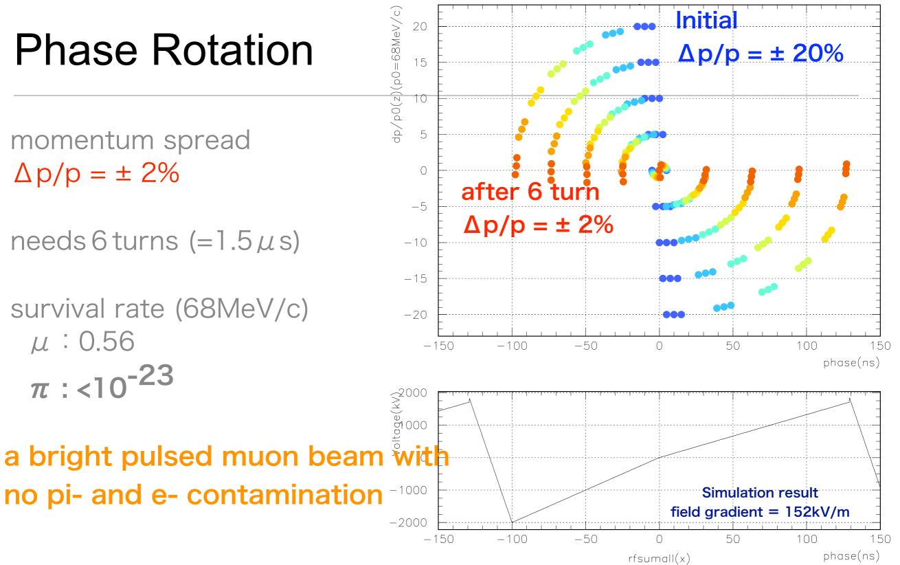
Shorter pulsed proton (<10ns) is required for phase rotation.
