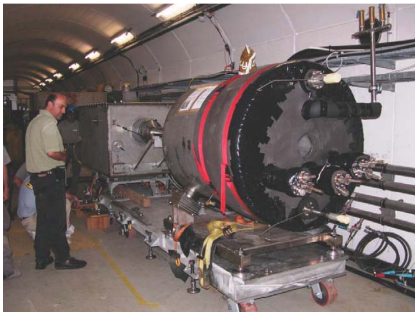
15-T solenoid and Hg jet installed in TT2A tunnel at CERN
