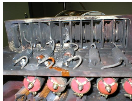
Siemens HVPS damaged HV cabling and diode bridge during high power tests
