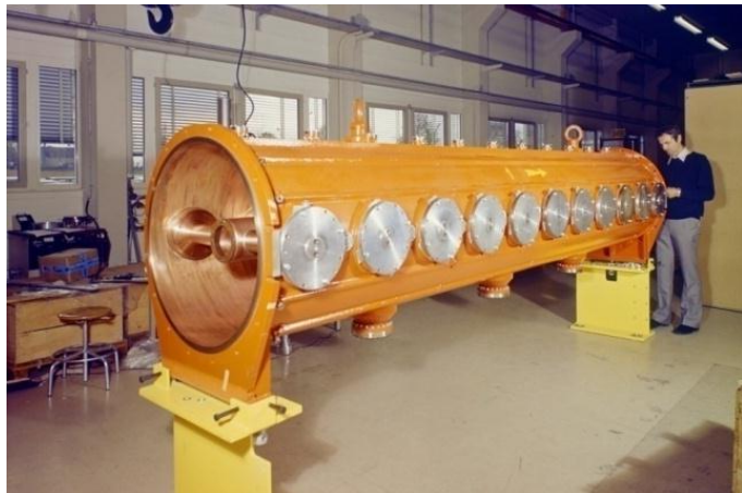
One section = 11 drift tubes
