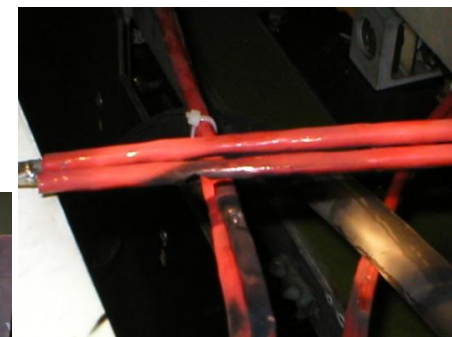
Siemens HVPS damaged HV cabling and diode bridge during high power tests
