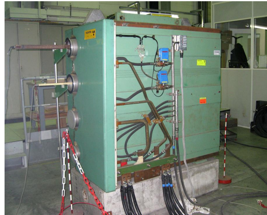
Booster main magnet undergoing tests for operation at 2 GeV
