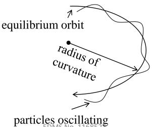
particles oscillating EDMS No. 1168522 around design orbits
