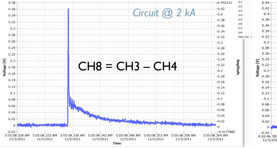
CH8 corresponds to the signal seen by the quench detector (all the inductive voltages are cancelled, only the resistive signal is seen, unless... Unless there are some signals on EE131 which could be seen as well: electronic artifact
