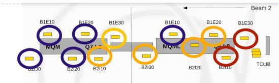
Two monitors in Q6 continuously in saturation. Four monitors in Q7 and 1 monitor in Q6 never reach saturation. Three monitors in Q6 and two monitors in Q7 eventually reach saturation. When saturated, the signals of these monitors can be reconstructed from reconstructed via B1E10.
