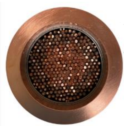
Subelement assembly 192 Cu/Nb-Ta filaments
