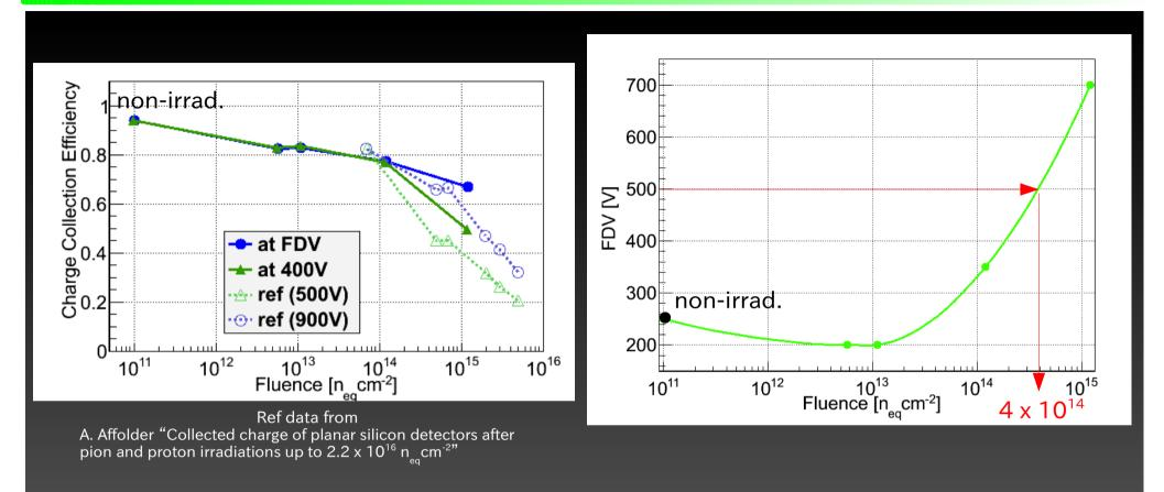
The CCE(solid line) is in good agreement with the data from  $\beta$ -ray tests(dashed line).
