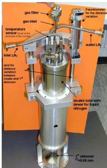
Supersonic jet gas target developed in GSI
