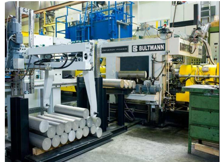
Induction heating of aluminium billets
