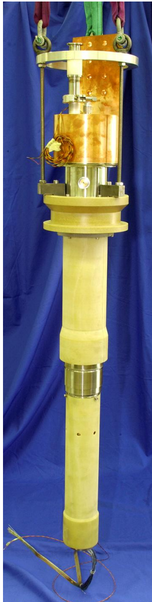
13 kA lead for LHC (photo CERN)
