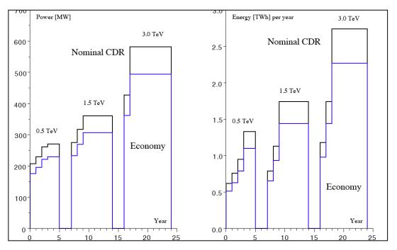
Other models can be envisaged (this is one out of many), and one should also keep in mind that reducing the instantaneous luminosity at the highest energies reduced both power and yearly energy, and finer energy scans might well be needed within one stage
