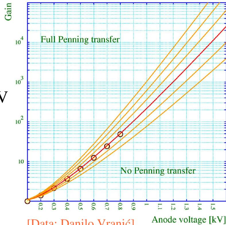
Gain vs Anode voltage (inner chamber)
